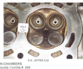
Picture H - Combustion chamber after P.i. treatment
