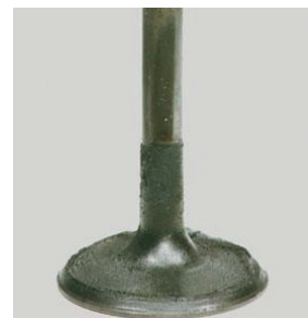
Picture E - Intake valve after P.i. treatment
