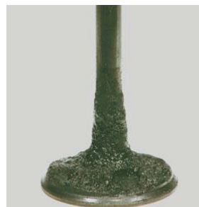
Picture D - Intake valve before P.i. treatment
